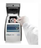
Place test disc in the **cobas b** 101 and close lid. The measurement starts automatically.
