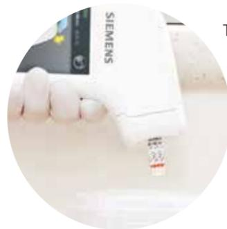
Test strip eject button reduces biohazard exposure.
